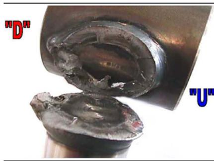
Rod weld breakage
