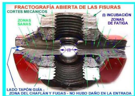
Stress crack in oil port
