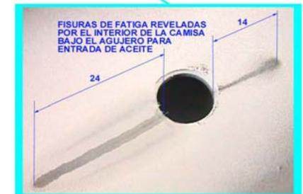
Stress cracks revealed by the inside bore, under the oil port hole.
